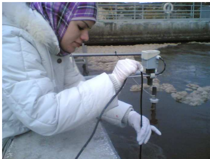
Figure. 7. The measurements of (DO) onsite to depth of 3.5m in aeration tanks
