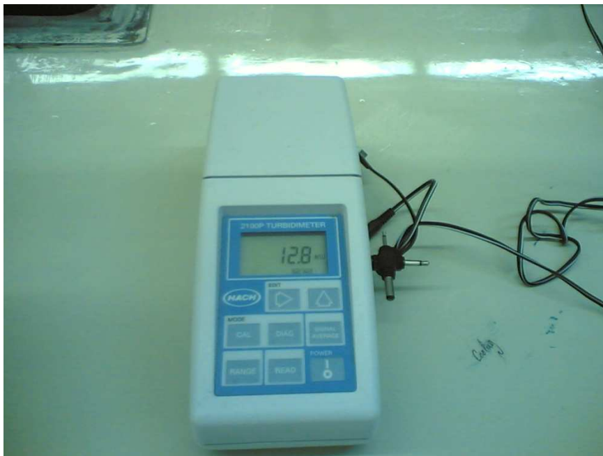
Figure. 8. Turbidity measurements in NTU unit
