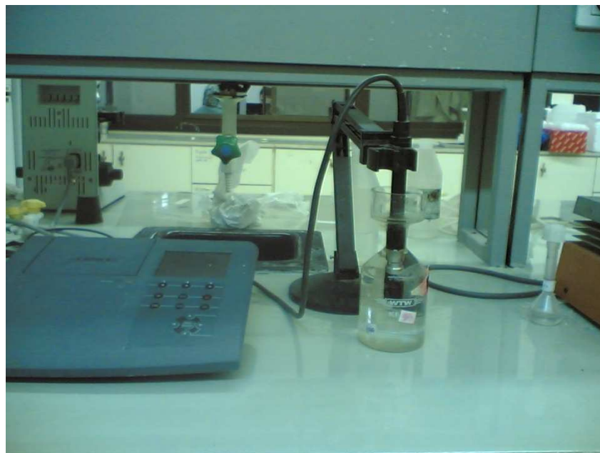
Figure. 10. The measurements of BOD 5 by Dissolved Oxygen METER
