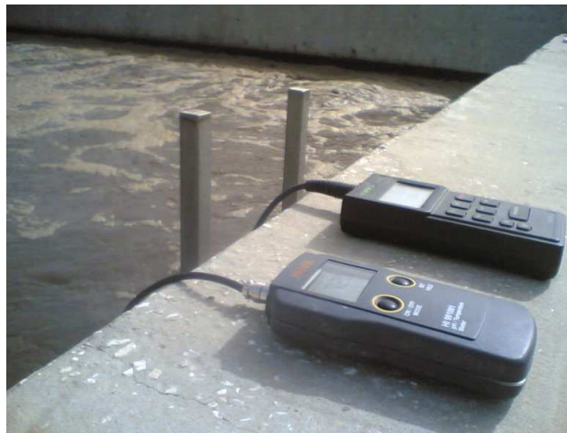
Figure 6.The measurements of T and pH value onsite in aeration tanks
